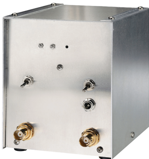
Figure 4 — The rear-panel switches select peak/average power readings and internal battery/external dc power. The BNC connectors are for the transceiver and load or antenna.
