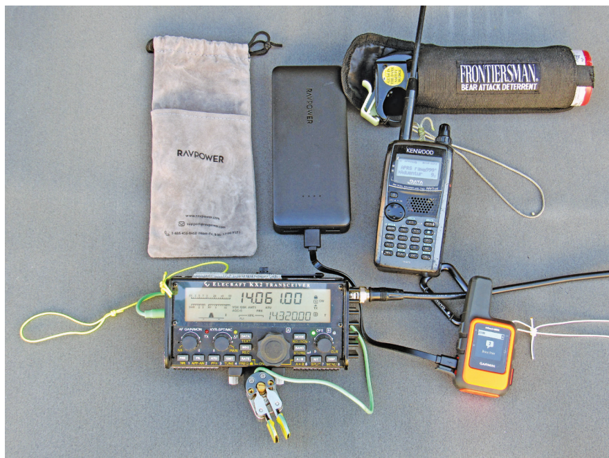
Figure 9 — N7RR's backcountry station includes an Elecraft KX2 for HF operation, a Kenwood TH-D72 dual-band handheld with APRS, RAVPower USB power bank, Garmin inReach Mini, as well as a canister of extremely effective bear spray to defend himself against North American predators like cougars and bears. [Margaret Prior, K7MWP, photo]
